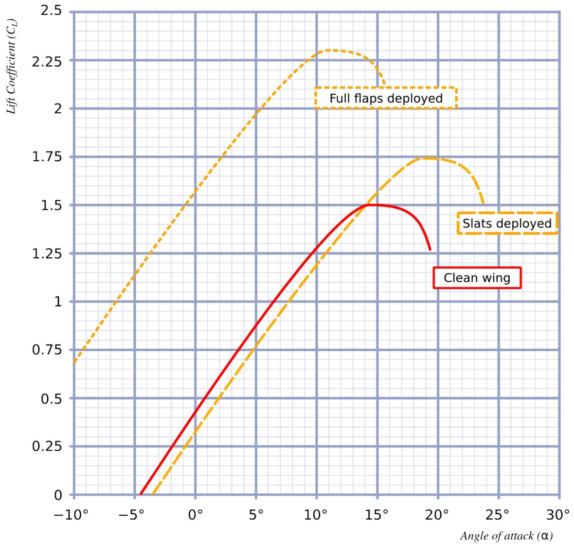
Figure 1.2: Lift coefficient as a function of angle of attack for the aircraft, as measured on a representative wind tunnel model.
