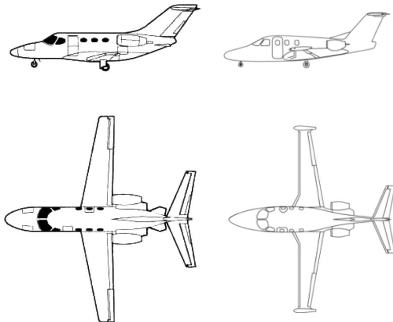
Figure 1.1: Three-view plans of the Cessna Citation Mustang (left) and Eclipse 500 (right), drawn approximately to scale.
