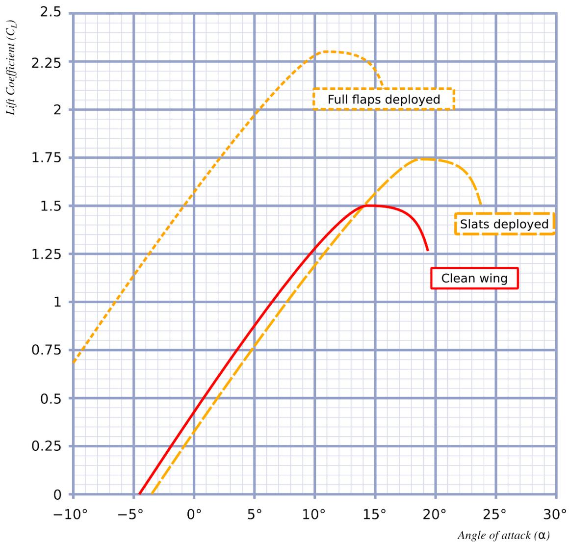
Figure 2.1: Lift coefficient as a function of angle of attack for the aircraft, as measured on a representative wind tunnel model.
